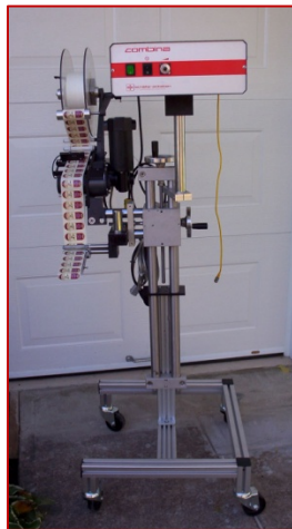
Top applicator Combina labeler with adjustable stand for conveyor use
