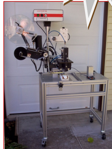
Tap on Combina labeler with table operator product positioning
